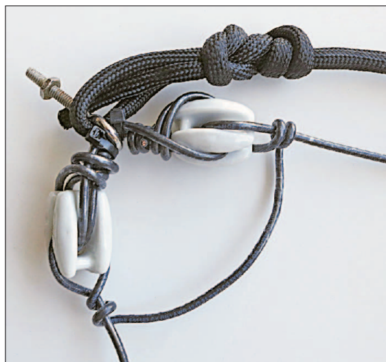
Figure 3 — Corner strain relief uses antenna rope and egg insulators.
